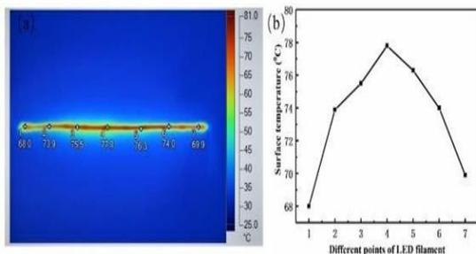
**Simulation results of LED filament**
