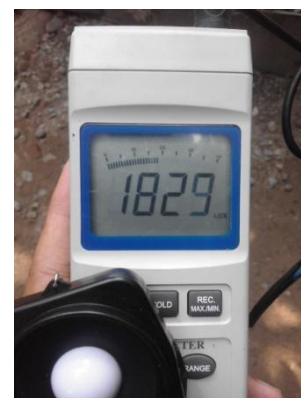
Figure 3. Light meter LX used in this experiment to estimate a large amount of sun intensity
