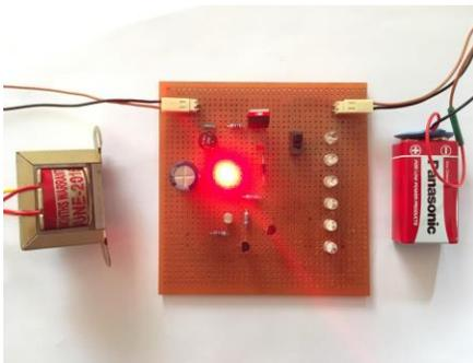
**Figure (18):** LED Output While Darkness Spread Over LDR
