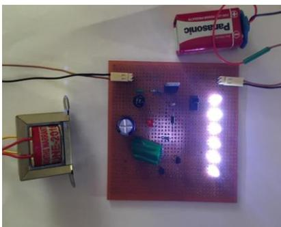
**Result:** The output of the LEDs is measured and tested battery backup is approx. 8 Hours. At the input of the battery the measured voltage is 4.5V through Zener Diode. Across Capacitor measured voltage is 12.15V DC and from calculated current is 12.15mA. Across Diode D2 voltage is 13.7V. This circuit can also be extended to a higher output voltage for which the charging voltage and the load
