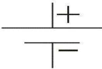
For Rechargeable battery, Nominal Voltage of Li-Ion battery is 3.7 Voltage. Standard capacity is 1950mAh. Charging voltage is 4.2V. Constant current 0.2C5A.
