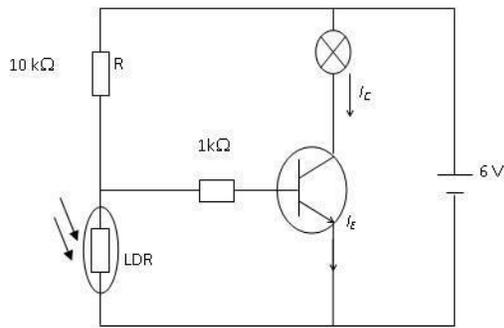
The circuit shown above shows a simple way of constructing a circuit that turns on when it goes dark. In this circuit the LDR and the other Resistor form a simple 'Potential Divider' circuit, where the centre point of the Potential Divider is fed to the Base of the NPN Transistor.
