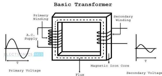
Figure (2): Step Down Transformer
